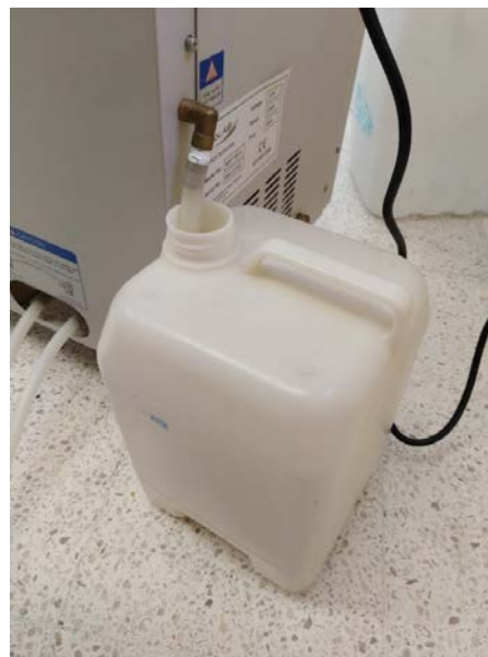
Steam outflow hose properly seated in water recollection bottle.
