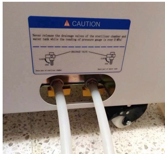
Main chamber drainage water valve (in the closed position).
