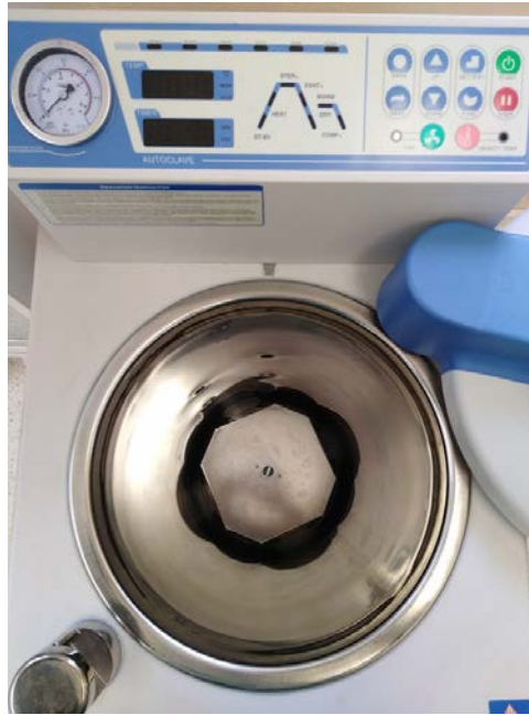
Main chamber floor-plate (octagonal plate in centre).
