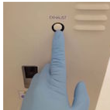
Exhaust purge valve.
