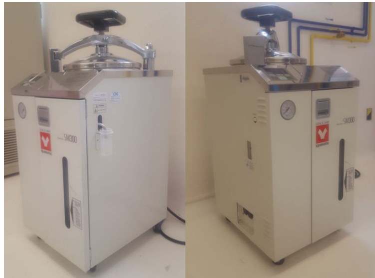
36 Litre Yamato SM300 autoclave/sterilizer used.
