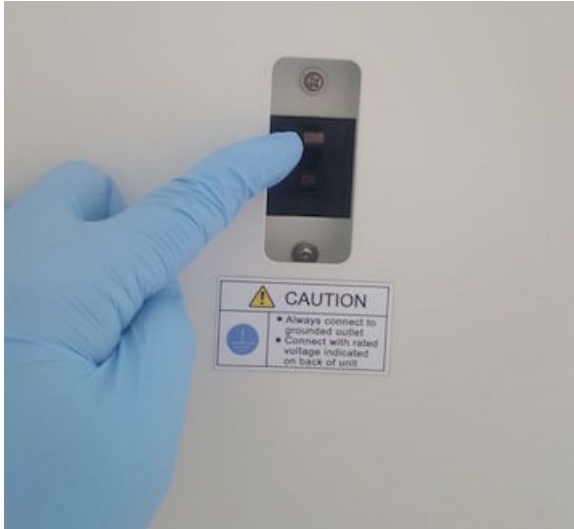
Thermomagnetic electrical switch.
