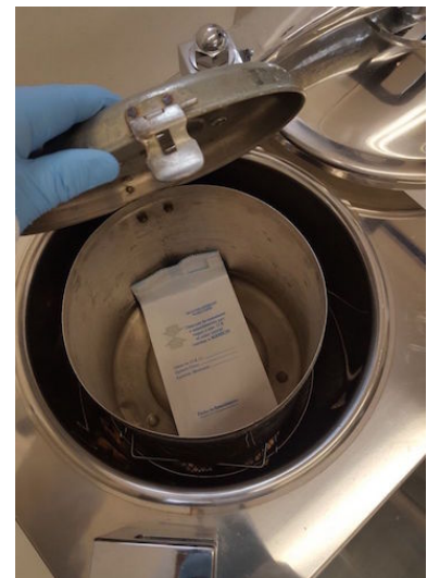
Autoclave container with carcass bag.
