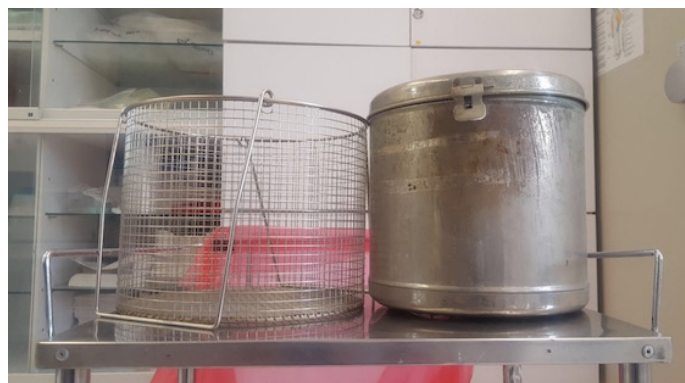
Wire mesh autoclave basket and autoclave metal container.
