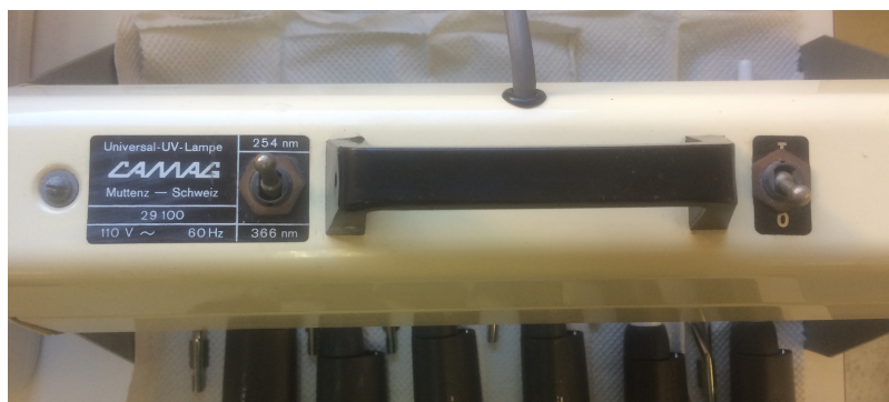
Camag universal UV light source set for 254 nm in the off (0) position.
